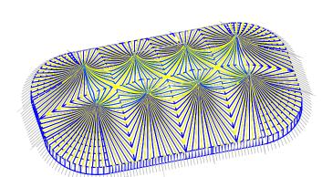
Wind speed = 42 m/s. Wind load = 0.5 Kn/m2
